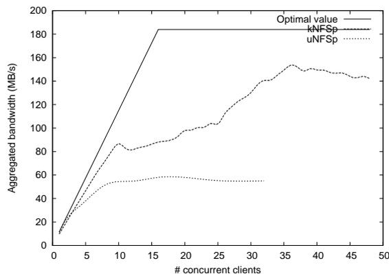
**Fig. 4.** Comparison user-mode server - kernel-mode NFSP server - 16 iods
