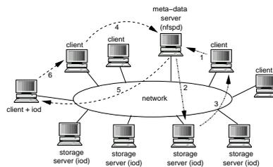
**Fig. 2.** Architecture of a NFSP system
