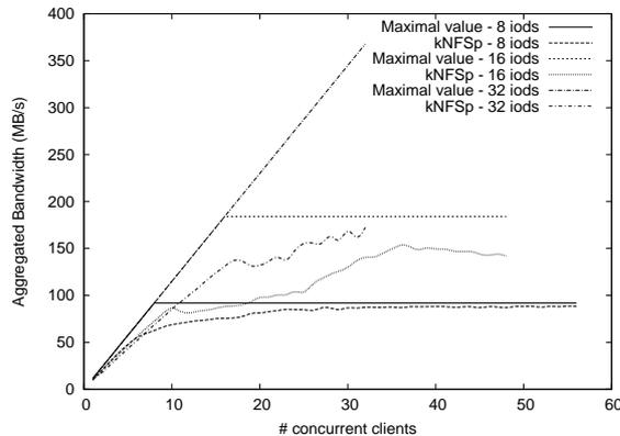
**Fig. 5.** Comparison user-mode server - kernel-mode NFSP server - with a varying number of iods
