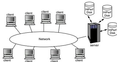
**Fig. 1.** Architecture of a NFS system
